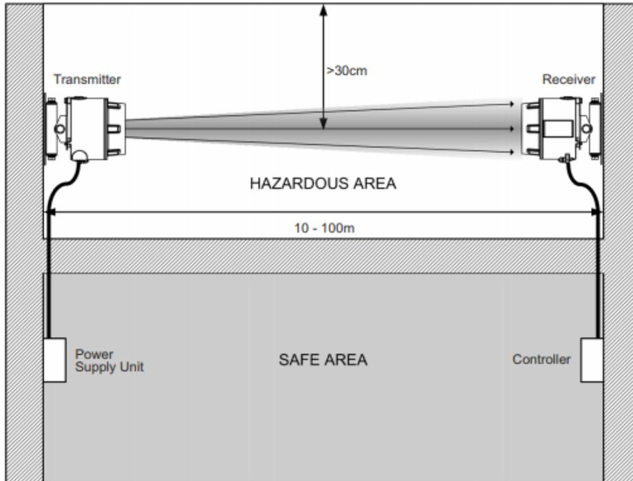
Only the ExD TX and ExD RX can be placed in the Hazardous Area.
