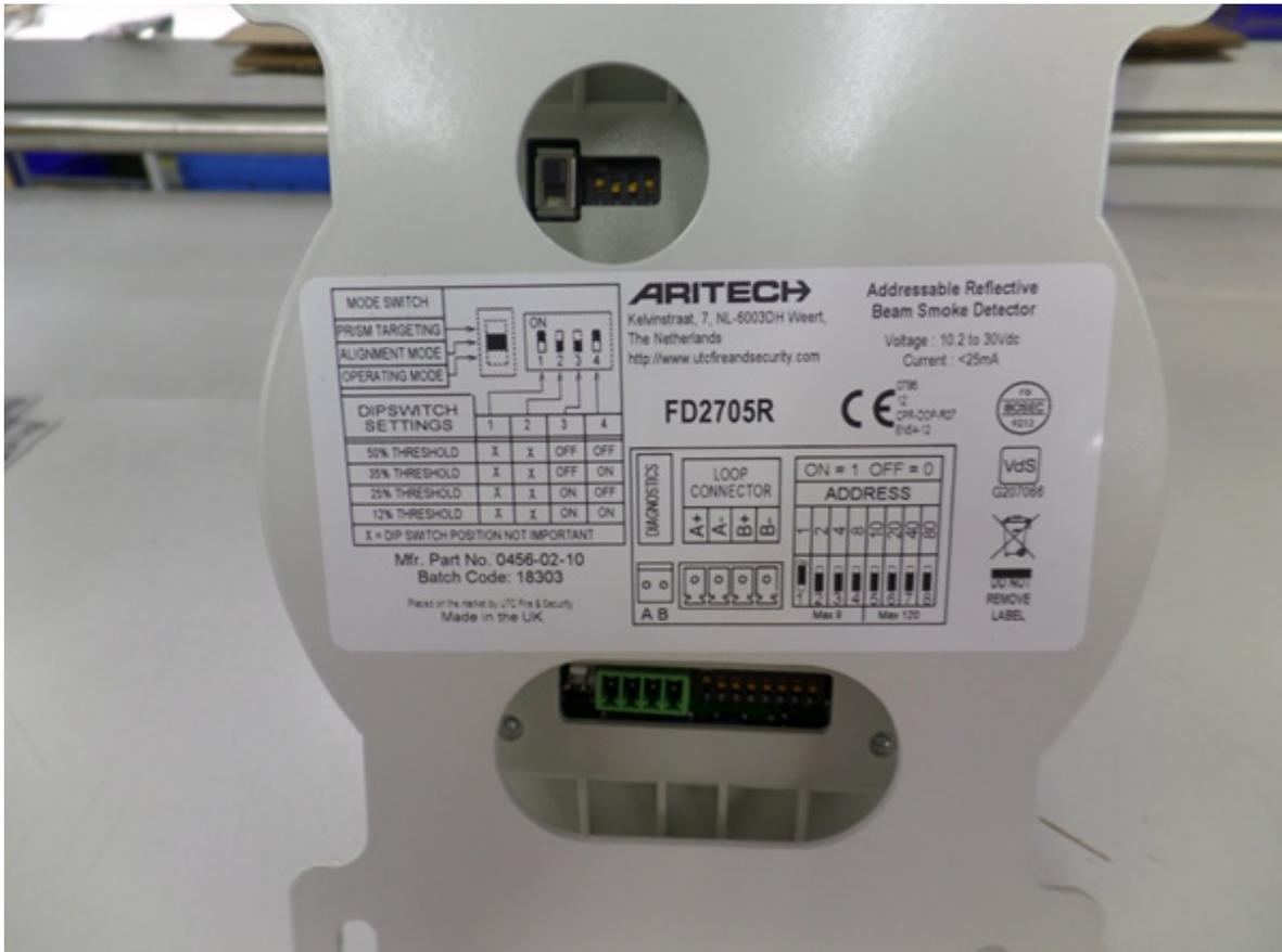
Prism targeting on AA 50/100Rs is different from the Standard 50/100Rs, but ultimately achieves the same thing. You will need to refer to the manual for each AA Beam as the procedure is not the same for all the AA 50/100Rs.
