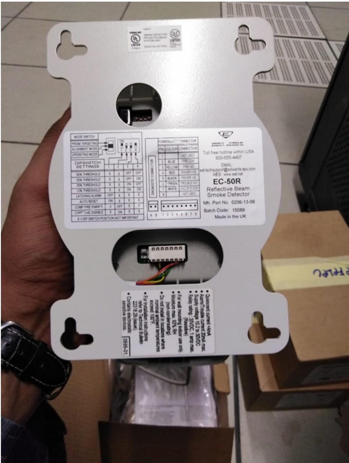
When the alignment has been completed (on both thumb wheels), set the switch to the bottom (run position). After 10 seconds, the Detector should be ready to test.
